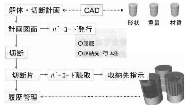
Fig.7 Outline of the Dismantling Engineering System applied to the Natural Uranium Conversion Facilities
