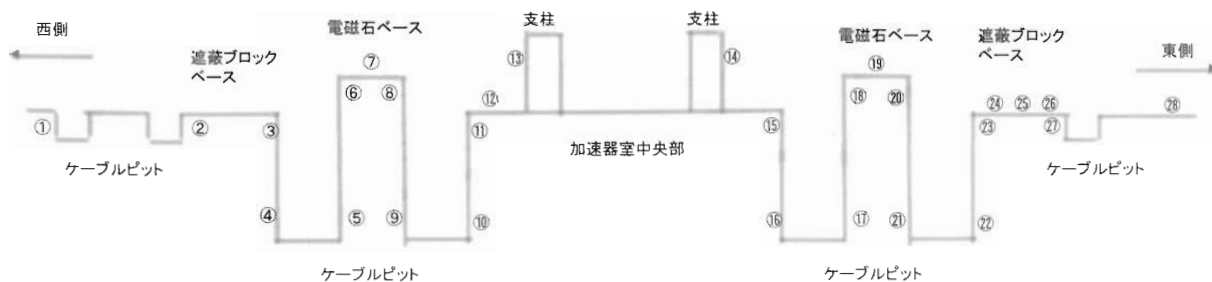
Fig.8 Measurement Points of Surface Dose Rate and Activity of Co-60 of the Crosscut of the Synchrotron Room.
